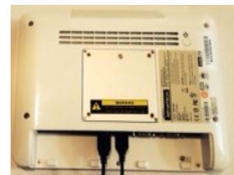
Figure 1. USB connections.
