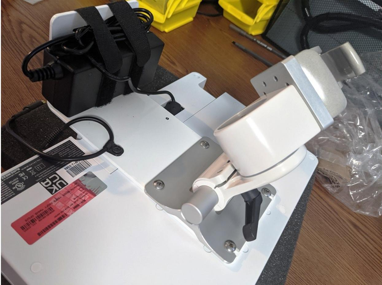
5.5. You can now use the pole clamp to attach the unit to the bedside pole.
