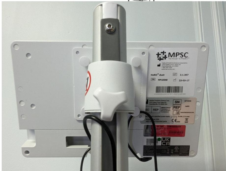
Step 4: Attach the HeRO monitor to the VESA mount. If necessary, adjust screw because monitor is too heavy or too light for mount.
