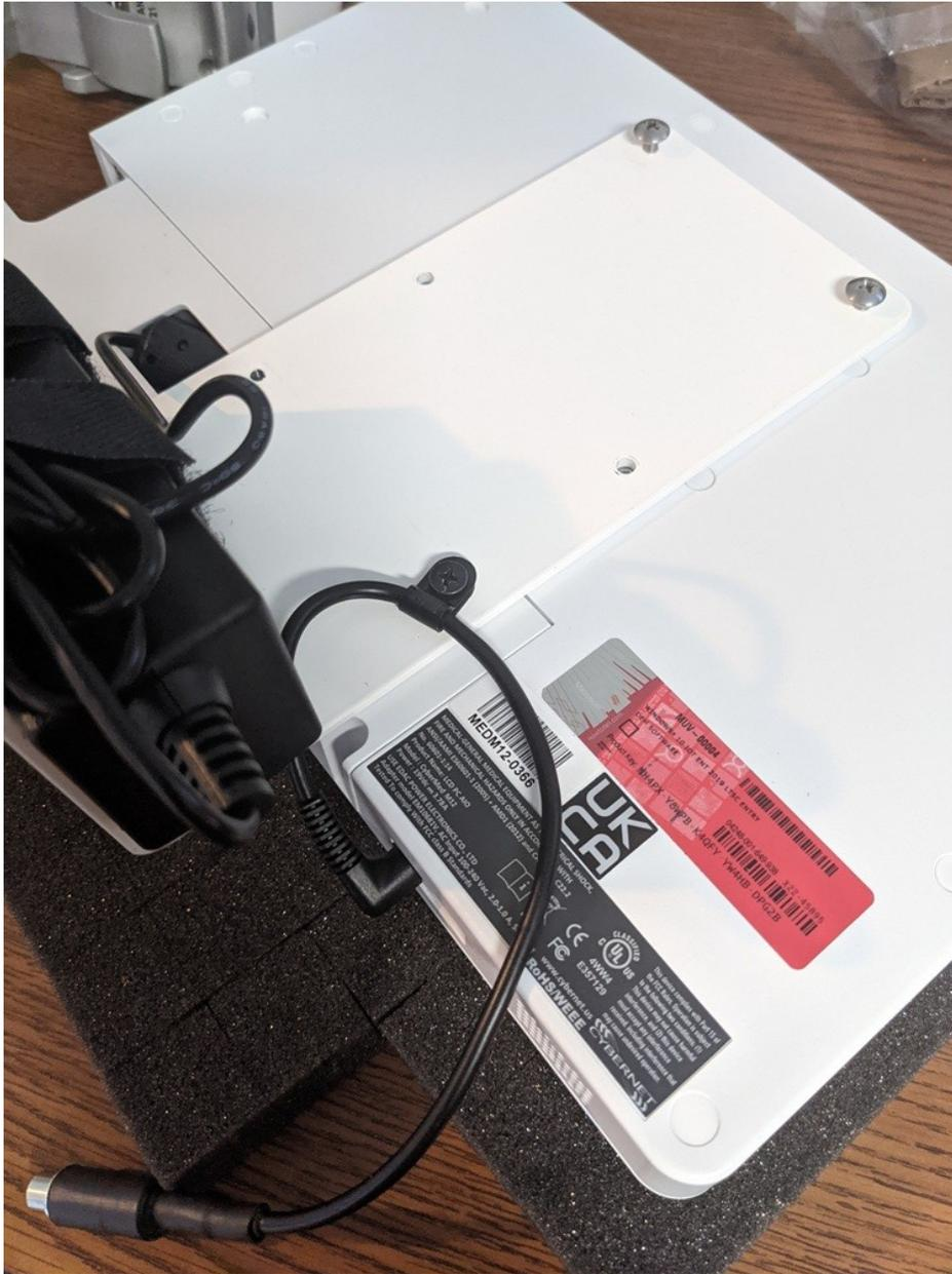
5.4. Attach the VESA mount to and power supply as shown.
