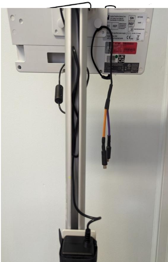
Step 5: Push the power cord in to the channel.
