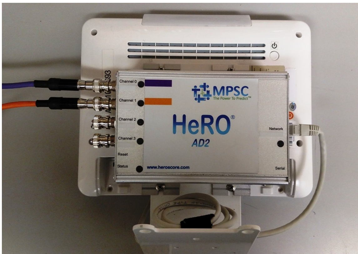
Figure 2b. HeRO duet cabling when using the HeRO Data Acquisition Device (AD2). The purple patient cable is inserted into the Channel 0 port, and the orange cable into the Channel 1 port. An Ethernet cable connects the HeRO Data Acquisition Device (AD2) to the HeRO display. HeRO solo cabling is identical except for the omission of the second, orange patient cable. Not shown, RS-232 installations omit the HeRO Data Acquisition Device (AD2) entirely.
